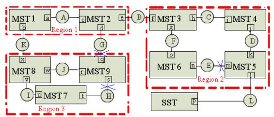
As shown in above figure, it is assumed that all ports of all bridges in the network have equal port path costs. The bridge identities of MST Bridge 1 and MST Bridge 9 are incremented at one time and the identity of the SST Bridge is the maximum.
