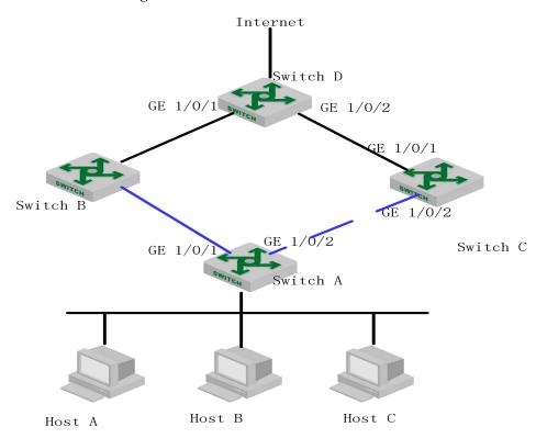
As shown in Figure 2-1, Switch A is configured with the Flex Links function for link redundancy backup. GE 1/0/1 is the master port and GE 1/0/2 is the slave port.
