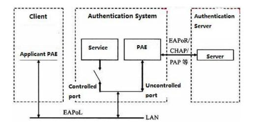
Figure 1-1 architecture of 802.1X
