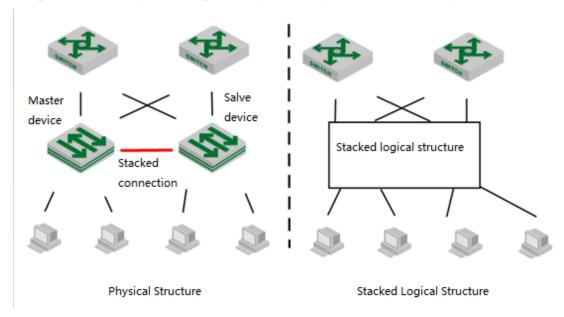
schematic diagram of stack networking applications
