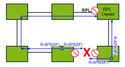
③As shown in Figure 1-3, when the link of the faulty device recovers, it sends RAPS (NR) packets to other devices in the ring to inform them that there is no local request. When the RPL owner receives the packet, it will block the port and send the R-APS (NR, RB) message again after some time. After receiving the packet, the other nodes will refresh the FDB entry. Later, the port of the faulty node will be restored to the forwarding state, and the ring will revert to the IDLE state (Figure 1-1)
