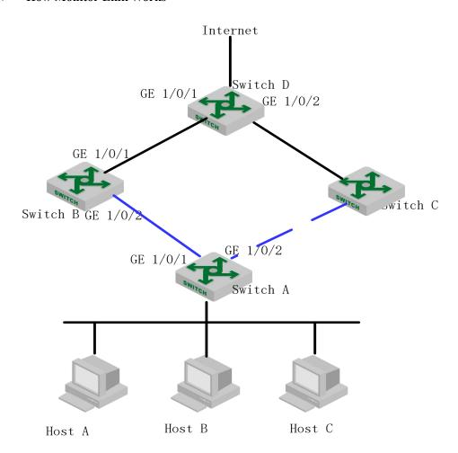
As shown above, a flexible link group is configured on Switch A to ensure reliable access to the Internet. In the figure, GE 1/0/1 is the master port and is in the forwarding state. GE 1/0/2 is the slave port.
