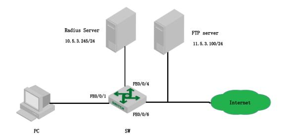
networking diagram for radius configuration example
