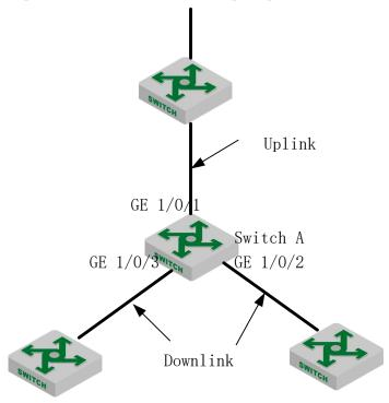
As shown in Figure 2-2, GE1 / 0/1, GE1 / 0/2, and GE1 / 0/3 of Switch A form a Monitor Link group.
