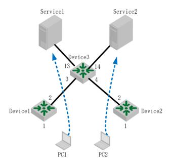
Network diagram of IP Subnet-Based VLAN
