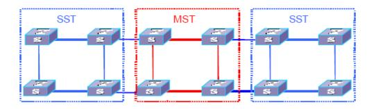
The switch in the red MST region uses the MSTP BPDU to exchange topology information. The switch in the blue SST domain exchanges topology information with STP / RSTP BPDU.
