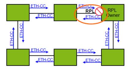
② When a node on the link detects a fault, it immediately blocks the faulty node and reports the fault message (R-APS (SF)) to all the other devices in the ring. After receiving the message, all other nodes refresh the FDB. The RPL owner port receives the fault message, and the recovery port is in the forwarding state. The ERPS ring enters the protection state. As shown in Figure 1-2:
