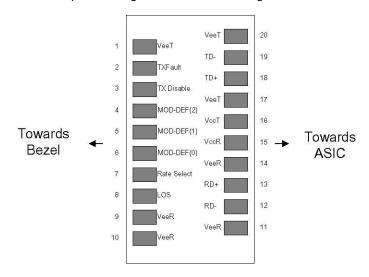
**Pinout of Connector Block on Host Board**
